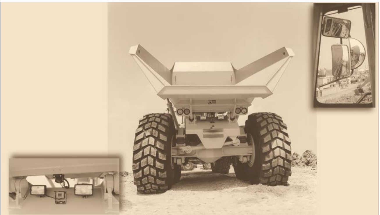
Figure 9 Photo montage of large dumper truck fitted with CCTV and mirrors to improve visibility from the driving position
